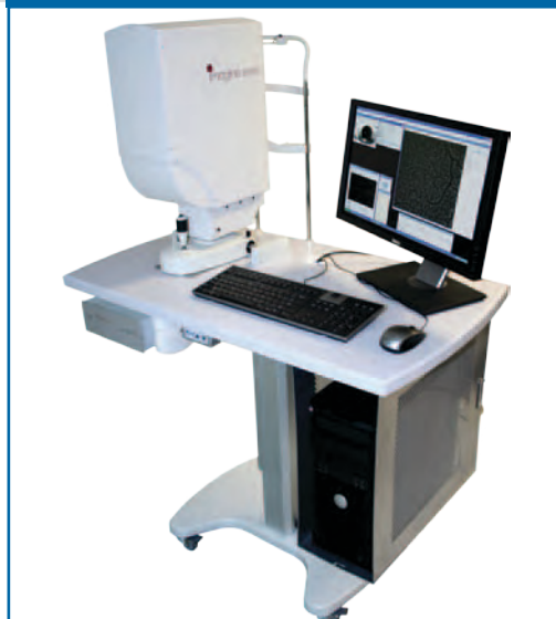
Figure 1: The rtx1 Adaptive Optics Retinal Camera.
